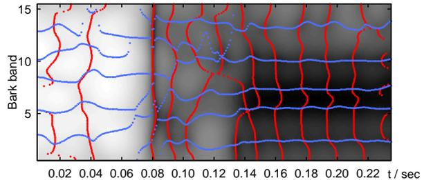
Figure 2: *PLP<sup>2</sup> pole locations.* The red points (which form vertical lines) are the poles for each of the FDLP temporal envelope estimates, and blue points (creating horizontal lines) show the poles for each of the spectral estimates from the conventional PLP stage.
