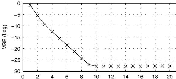
Figure 3: Mean-squared differences between the 28,800-point log-magnitude surfaces obtained in successive iterations of the PLP<sup>2</sup> approximation.
