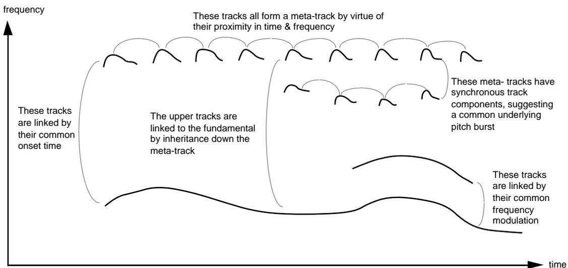
figure 3: diagram of grouping principles applied to tracks
