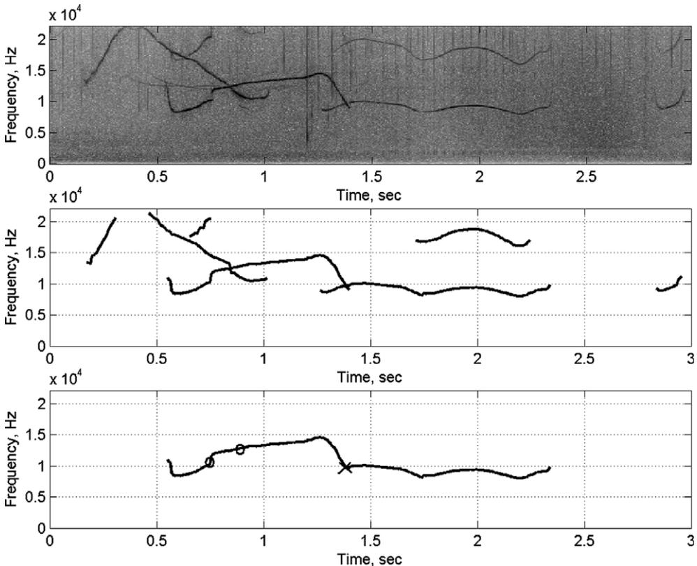
Fig. 6. Overlap example. Top row: original spectrogram depicting multiple calls. Middle row: extraction of calls. Bottom row: example calls. Circle indicates correct connection;  $\times$  indicates false connection.
