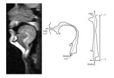
Discrete approximation as varying-diameter tube
