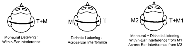
FIG. 1. Three configurations of the cocktail-party effect that isolate the effects of within-ear and across-ear interference. The left panel shows a monaural version of the cocktail-party task that produces only within-ear interference between the target talker T and the masking talker M. The middle panel shows a dichotic version of the cocktail-party task that produces only across-ear interference between talkers T and M. The right panel shows a hybrid version of the cocktail-party task that produces within-ear interference between T and M1 and across-ear interference between T and M2.
